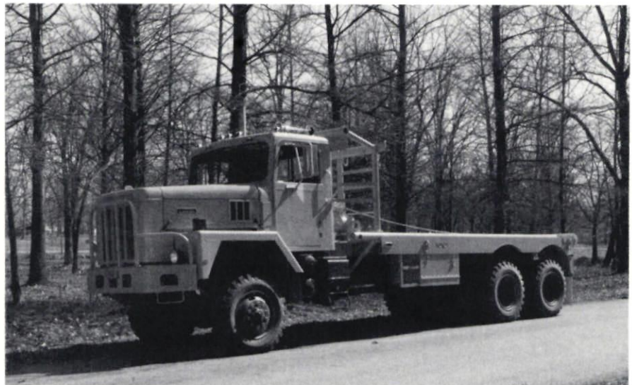
US oilfield equipment to PRC: International Harvester's 5000 Paystar INTERNATIONAL with special body and winch for use in oilfields.
