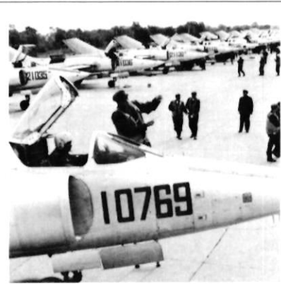
The Q-5 is an adaptation of the MiG-19 (or Chinese F-6) fighter with an extended nose bay—although China apparently lacks the sophisticated radar to put there—and air intakes moved to the side of the fuselage.
