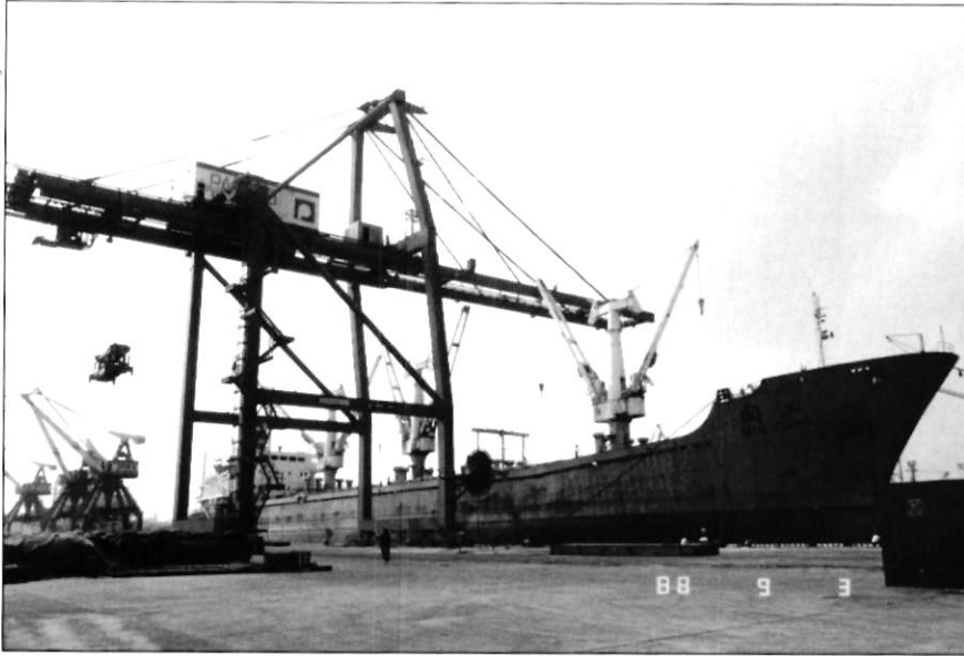
Key foreign equipment purchases have done much to improve Chinese ports. These container gantry cranes, built by a Chinese factory under license from Paccoco, were installed in late 1988 at the port of Dalian.
