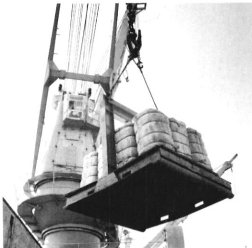
Two cargo boards are lifted from the hold using a double-robot.
