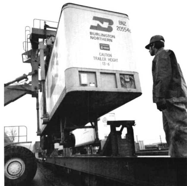
A railroad trailer is loaded onto a Chicago-bound railcar chassis at Burlington Northern's yards.
