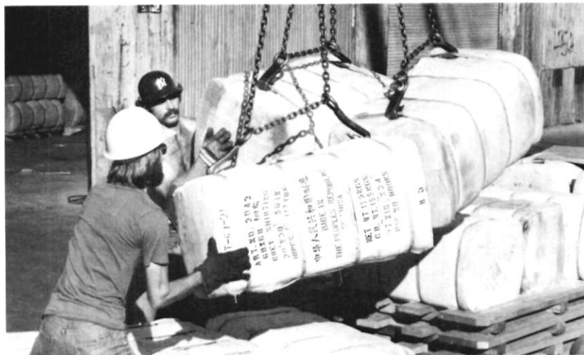
Bales are lifted from the hold using chine hooks and are loaded onto a cargo board on the deck.
