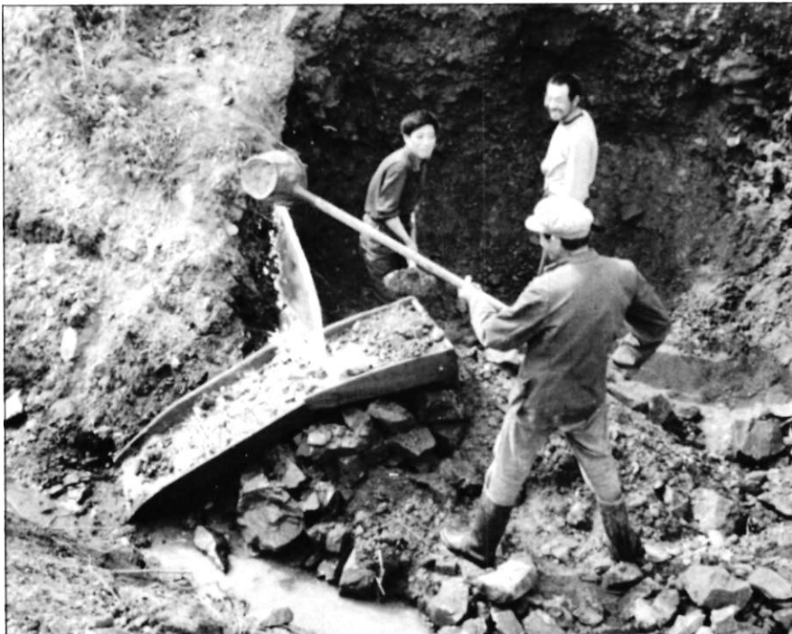
Peasant prospectors use a sluice box to extract gold from ore dug near Handaqi township in Heilongjiang Province.
