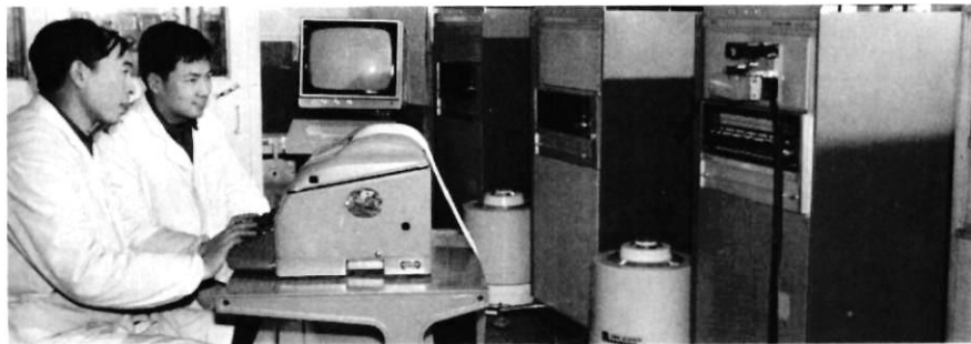
This DJS-130 digital computer, produced by the Suzhou Radio Factory, has an average speed of 500,000 operations per second.
