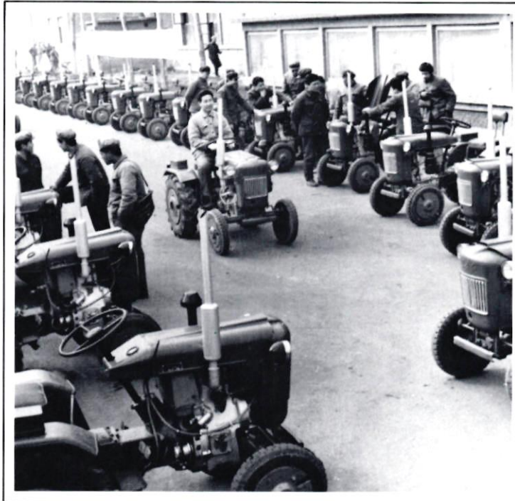
The 12 hp tractor made by the Xiangtai Tractor Plant.
