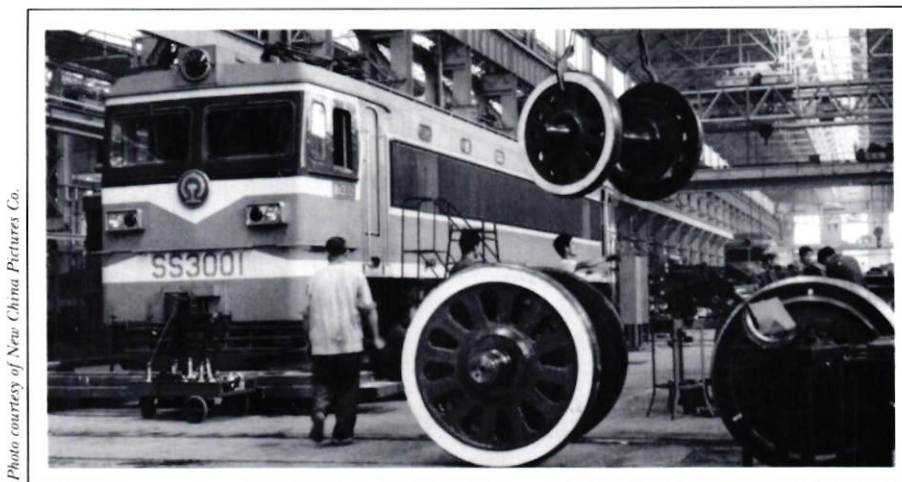
Shaoshan 1 electric engines being assembled at Zhuzhou's Tianxin Rolling Stock Plant, China's only electric locomotive manufacturer.
