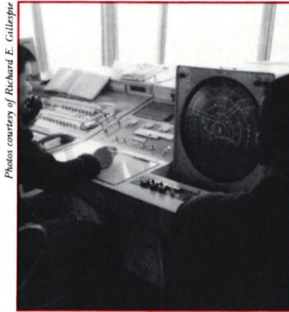
Air traffic controllers in the Beijing tower use approach control radar supplied by Thomson CSF.
