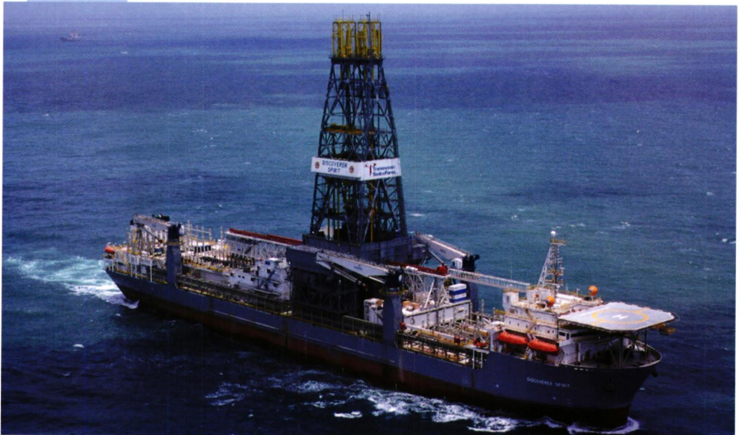
The ultra-deepwater drillship, Discoverer Spirit , drills in water depths up to 10,000 feet.
